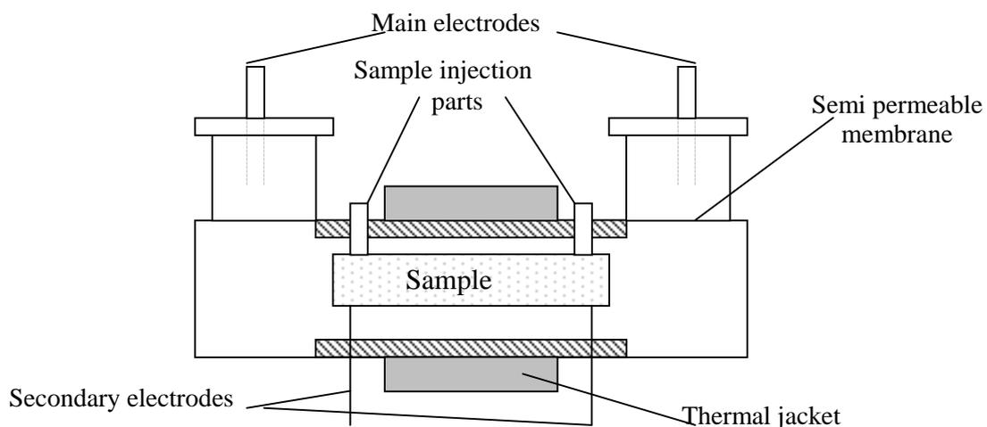
**Figure 4.2.:** Schematic diagram of the capillary electrophoresis cell for the zetasizer 3000.
