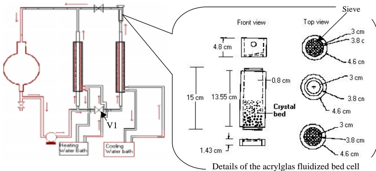
**Figure 4.1.:** Fluidized Bed Experimental Setup.
