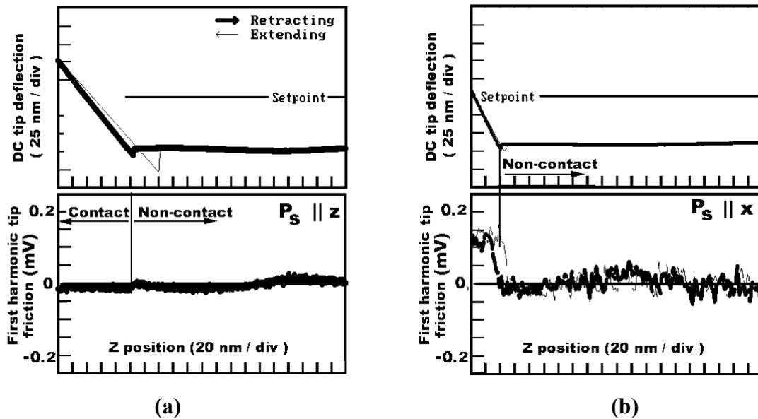
**Figure 15** First harmonic component of the x-deflection signal (lower plots) versus z-position of the scanner: **(a)** above a domain with polarization perpendicular, and **(b)** above a domain with polarization parallel to the sample surface (BaTiO<sub>3</sub> single crystal). The upper plots show the tip-to-sample contact position. Above the sample, in the non-contact region, the x-deflection signal is always zero.
