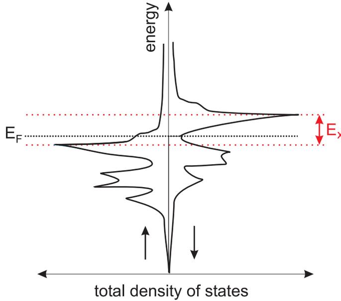
Figure 2.1: Total density of states of bulk Fe showing the exchange splitting by the amount  $E_x$  between majority electrons ( $\uparrow$ ) and minority electrons ( $\downarrow$ ) [42]. The Fermi energy is indicated by  $E_F$ .
