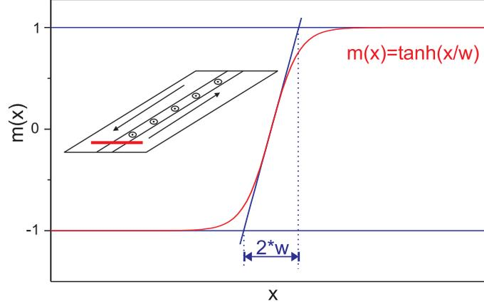
Figure 2.2: A magnetic line profile calculated for a  $180^\circ$  bulk wall. The line profile is a  $\tanh$ -function and the width of the domain wall is given by  $2w$ . In the inset, the underlying magnetic configuration is shown.
