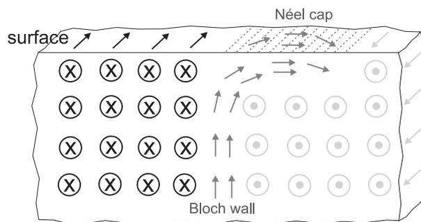
Figure 2.3: Schematic representation of the transition between a bulk Bloch wall and a surface Néel wall. The Bloch wall is running vertically through the center of the image and is terminated into a Néel cap at the surface. Crosses and dots correspond to magnetization vectors pointing in and out of the image plane.
