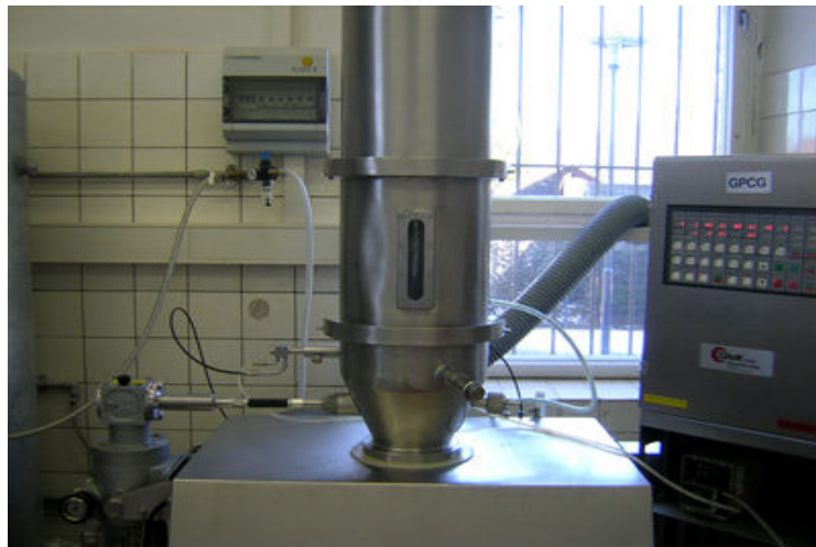
Fig. 2.1: Fluid-bed granulator (GPCG 1, Glatt, Germany)
