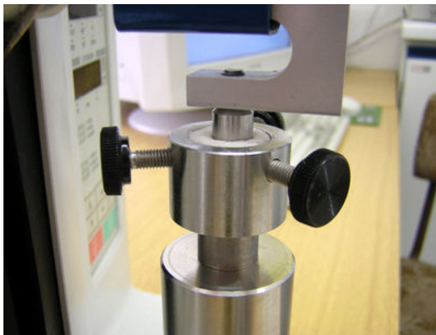
Fig. 3.6: Measurement of adhesion by texture analyzer
