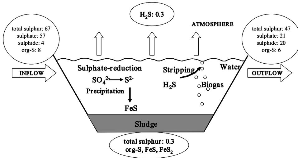
Figure 3 Annual mass balance of sulphur in an anaerobic pond; load expressed in kg S d<sup>-1</sup> (Paing et al., 2003)
