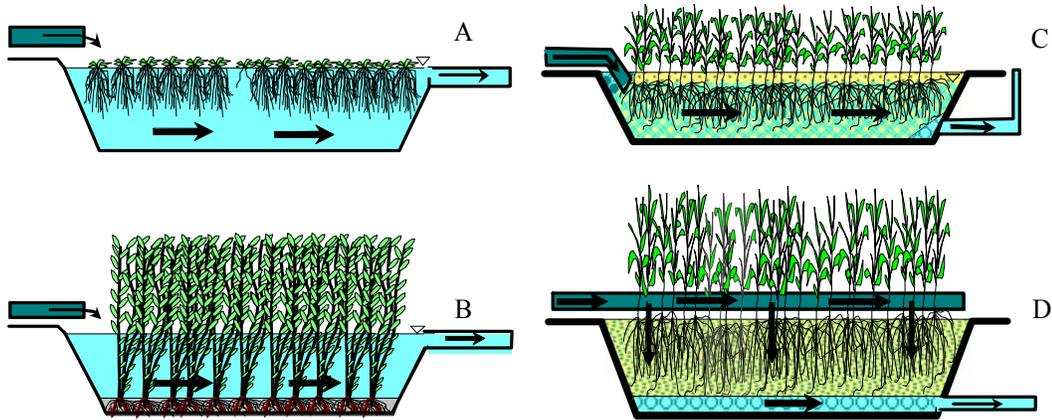
Figure 4 Pond/wetland systems for wastewater treatment (A, pond with free-floating plants; B, horizontal surface flow wetland or pond with emergent water plants; C, horizontal subsurface flow wetland; D, vertical flow wetland).
