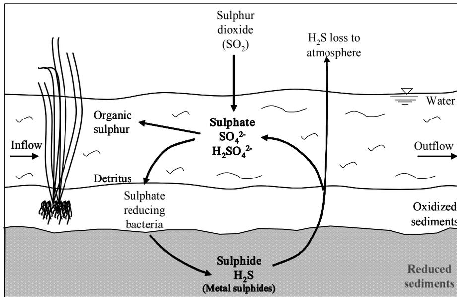
Figure 1 Typical wetland sulphur cycle.
