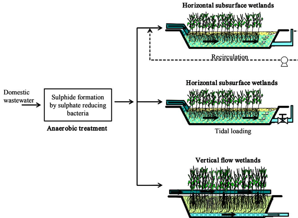
Figure 8 Possibilities for limiting the sulphide intakes to constructed wetlands.
