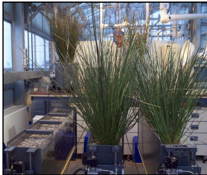
Figure 16 Experiment set up of the laboratory scale subsurface horizontal wetlands: W1 (unplanted), W2 and W3 (planted).
