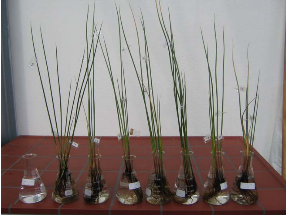
Figure 9 Experimental set up of the sulphide toxicity test of J. effusus after 50 days.
